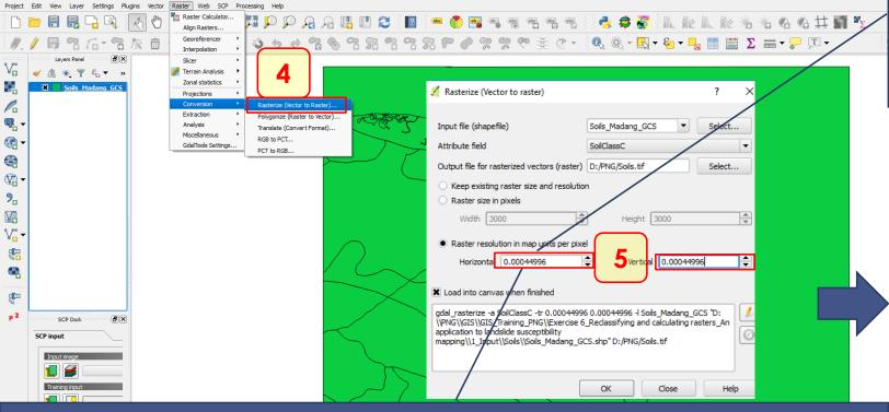
When defining raster pixel resolution, value will depend on layer's coordinate system e.g. in terms of meters if using projected system, or in degrees if using geographic coordinate system (1 degree = 111120 meters)
